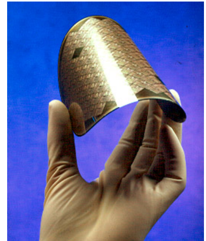
Ed Korczynski worked with 50µm thin silicon for TSV in 1999.
